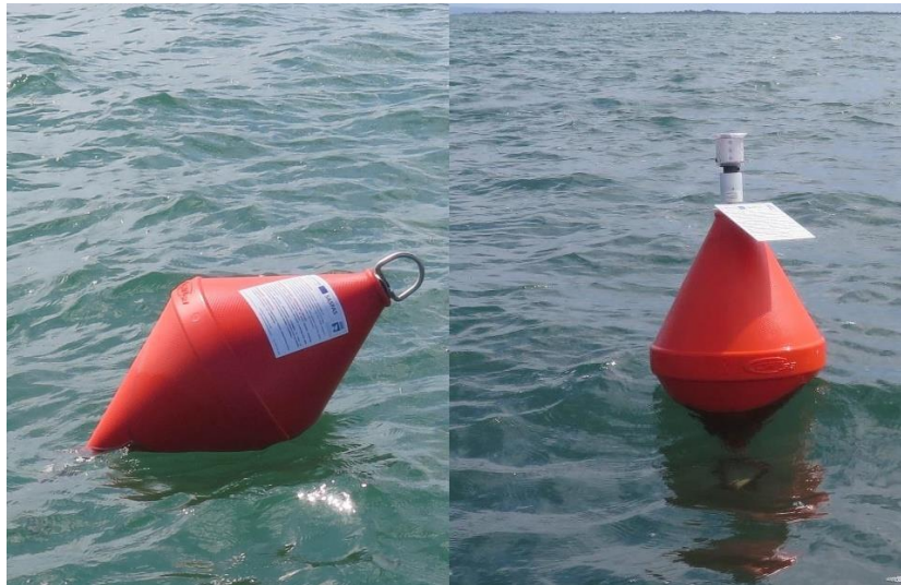
Figure 4-12. Buoys positioned at Monfalcone, in Panzano bay. On the left, an ordinary buoy and, on the right, a corner buoy, with lighting device.
