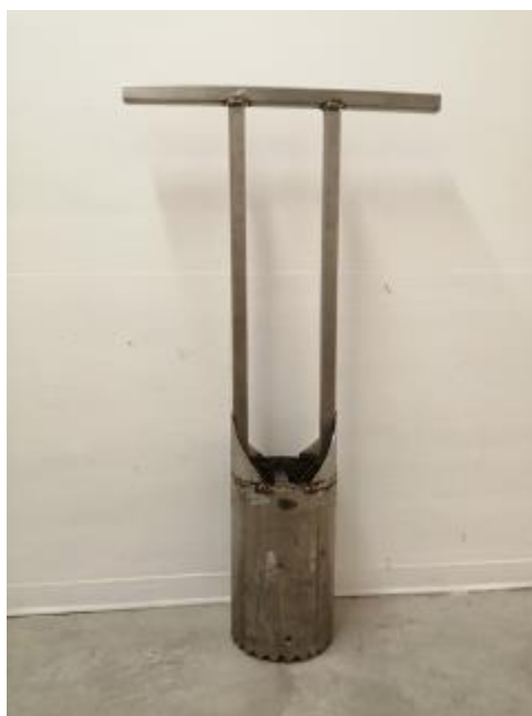
Figure 3-8. A typical steel core drill as the ones used to extract C. nodosa sods from the donor site to transplant them in the acceptor sites.
