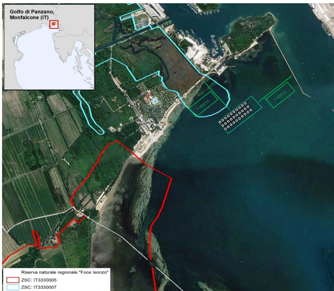
Figure 4-10. Photo-plan of the project area, in the Bay of Panzano. The polygon outlined in green represents the laying area of the buoy field that meets the criteria of distance from the coasts and harbour breakwater. The 30 white circles represent roughly the position of the 30 installed mooring buoys.
