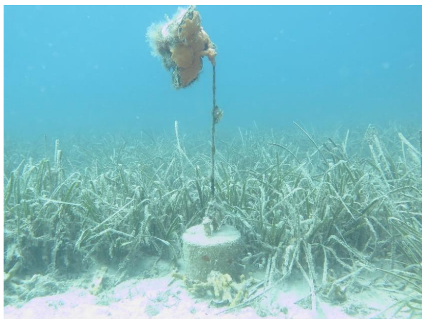
Figure 5-21. A balise is visible after a year of stay at the sea-bottom, partially colonized by fouling. A reasonable stable condition of the lower limit can be inferred. Their disappearance or overturning near the limit may also suggest the presence of trawling pressure or anchoring.
